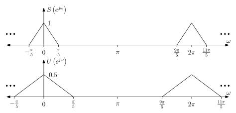
In order to minimize the order of H(z) its transition bandwidth must be as large as possible. Therefore, the passband frequency is  $\omega_s = \frac{\pi}{2}$ . The stopband frequency is  $\pi$ . Following gives the frequency response of H(z) and the signal v[n] and  $\hat{s}[n]$ .
