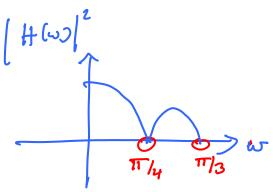
The role of modulation codes is crucial to examine  $S_{xx}(w)$  so that it does not Coincide with a spectral null of  $[H(w)]^2$
