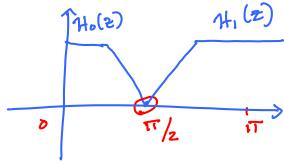
of Stop band attenuations are sufficiently large sufficiently large is not predominant Severe attenuation @ IT/2.
